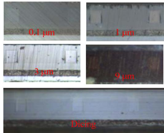
**Figure 7.** Waveguide terminal surface image.
