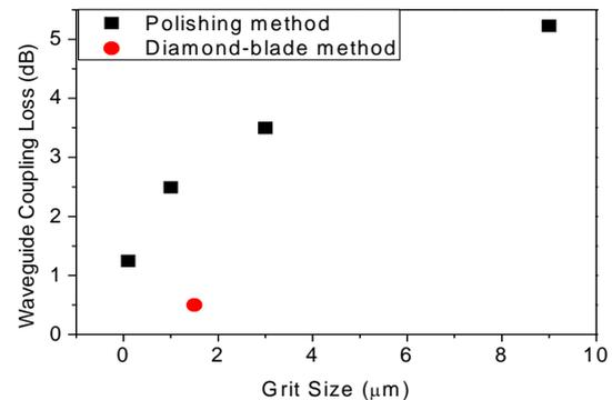
**Figure 8.** Waveguide coupling loss between different waveguide terminal surfaces.
