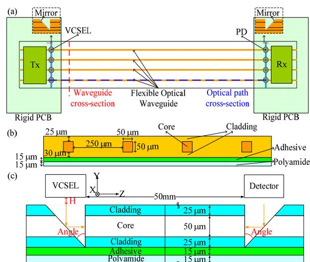
**Figure 1.** (a) FOW typed EPCB top view. (b) Waveguide cross-section on the inputs. (c) Optical path in cross-section.
