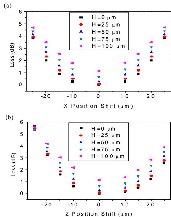
Figure 3. (a) X position and (b) Z position shift tolerance calculation.
