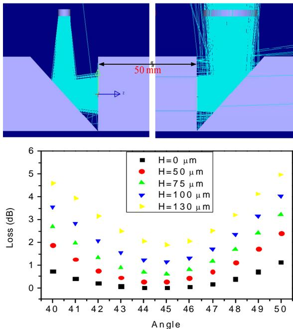
Figure 2. Mirror angle tolerance calculation.
