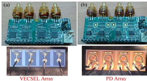
**Figure 9.** (a) Transmitter and (b) receiver active electro-optical module with 4-channel VECSEL array and PD array respectively.
