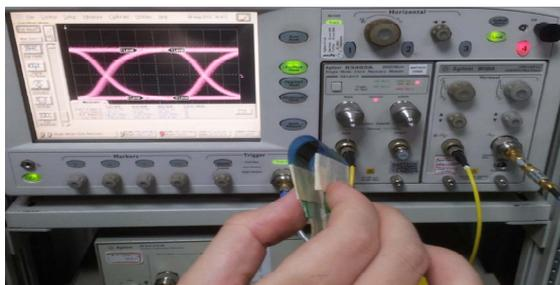
**Figure 11.** 2.5 Gb/s eye-diagram per channel for the FOW typed EPCB at 180° bend. from 44° to 46° was less than 0.5 dB. The diamond-blade method was applied and implemented on the 45±1° mirror. The waveguide coupling loss was discussed by different waveguide terminal surfaces. The diamond-blade method could provide smooth surface
