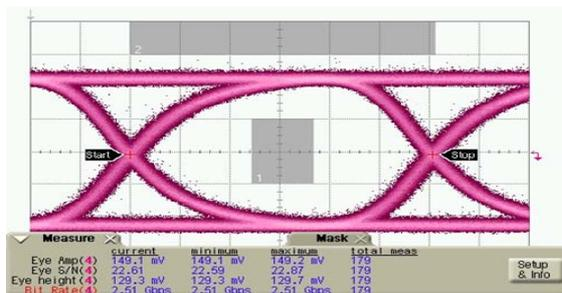
**Figure 10.** 2.5 Gb/s Eye diagram for one channel polymer waveguide.
