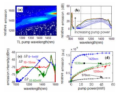
Figure 3. (a) Tunable laser based excitation-emission spectra, (b) the emission spectra of a short section of Bi Er co-doped fiber when increasing the 830nm pump power, (c) the increased emission between different pump powers, and (d) the relationship between the pump power and the emissions at different wavelengths.
