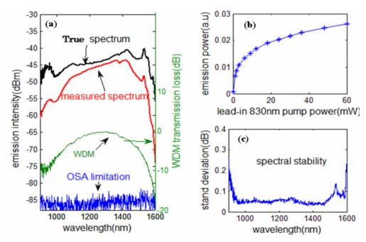
Figure 2. (a) Broadband emission, (b) the total emission power changed with the pump power, and (c) the standard deviation of the broadband spectrum.
