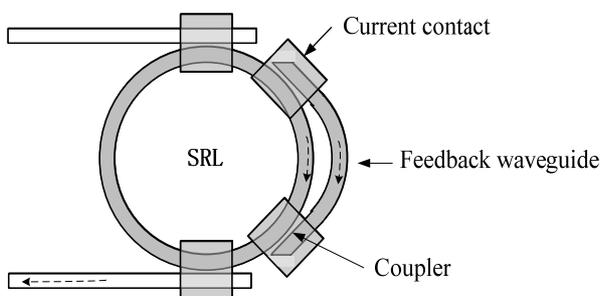
**Figure 1.** Schematic illustration of a SRL with a feedback waveguide.
