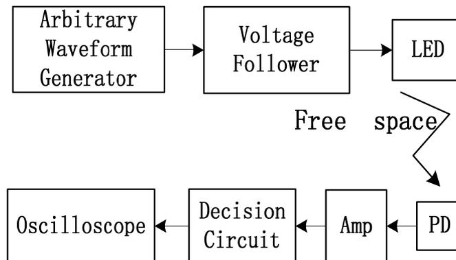
Figure 6. Testing block diagram.
