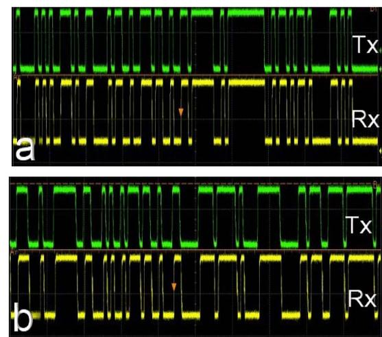
Figure 9. Captured data waveforms after decision circuit at (a) 1 Mbit/s data rate, (b) 2 Mbit/s data rate.
