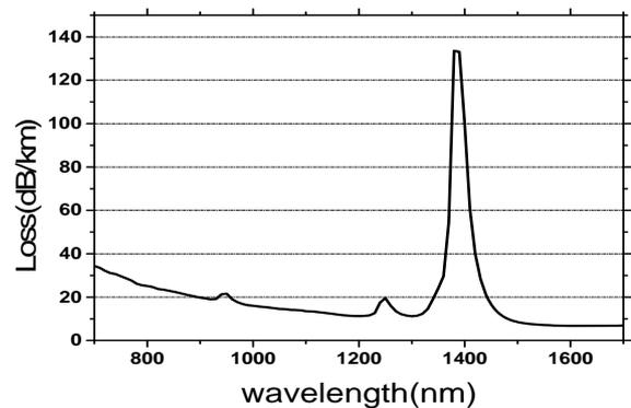
Figure 4. The attenuation spectrum of seven-core PCF.
