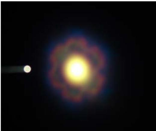
**Figure 7. Beam profile of SCG after the seven-core fiber.**
