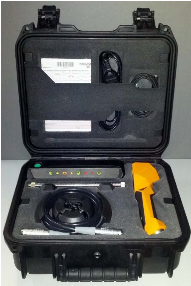
Figure 1. Photo of SF 6 Laser Gas Test.
