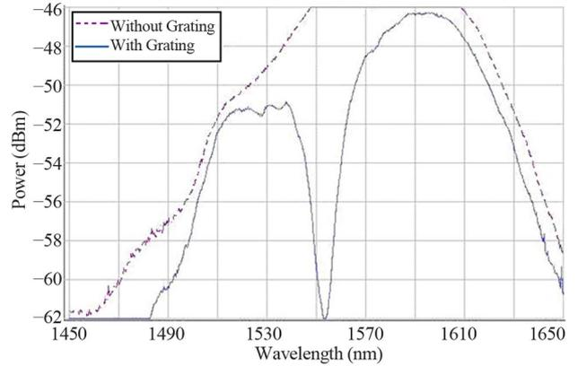
**Figure 2. Spectral response of MLPFG in MSM fiber structure.**
