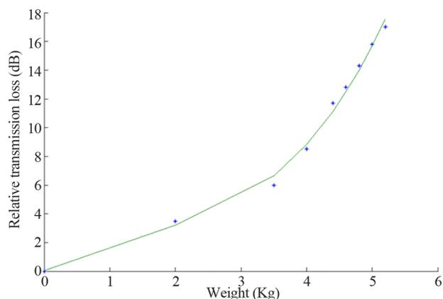
**Figure 4. Response of grating to external applied pressure.**
