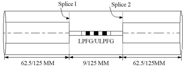
**Figure 1. Multimode-Single mode-Multimode (MSM) Fiber Structure.**
