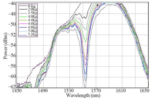
**Figure 3. Complete transmission spectrum of MLPFG in MSM structure ( $\Lambda = 600 \mu\text{m}$ ) with different pressures**
