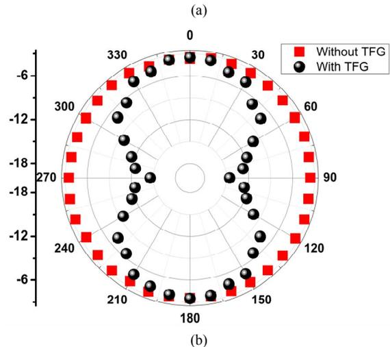
**Figure 2.** (a) The PDL measurement of *S*- and *P*-polarized light from the 15 mm long 45°-TFG, showing a PDL of ~13 dB; (b) Polarization distribution figure: Red square dots showing 0 dB PDL as measured from a virgin fiber; Black circle dots showing a near-8 figure shape measured from the 15 mm long 45°-TFG.
