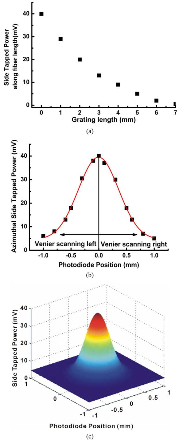
Figure 4. (a) Measured side-tapped out power along the length for the 9 mm 45°-TFG; (b) Measured power distribution in azimuthal direction, showing a Gaussian profile; (c) Re-plotted measured power distribution in azimuthal direction in 3-D.
