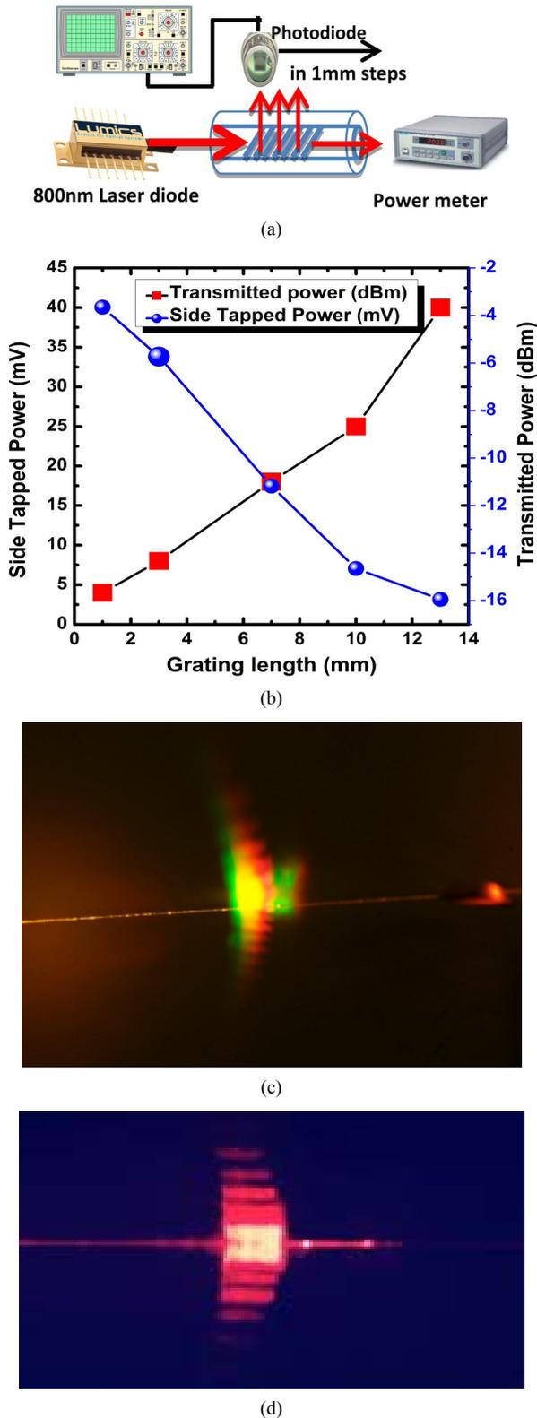
Figure 3. (a) Experimental setup for power tapping measurement; (b) The side-tapped (circle) and transmitted (square) power from the fabricated five 45°-TFGs of different lengths; (c) Images of side-tapped out light when launched with a white (SuperK) and (d) Red light, respectively.
