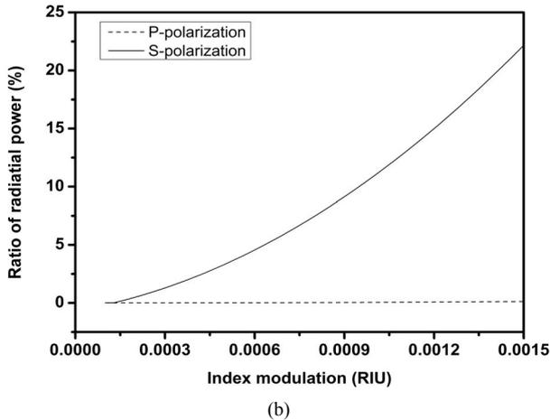
**Figure 1.** (a) Vector phase matching condition for a 45°-TFG; Inset: microscopic image of a UV-inscribed 45°-TFG; (b) simulated ratio of radiation power of S- (solid line) and P-polarization (dash line) for a 45°-TFG.
