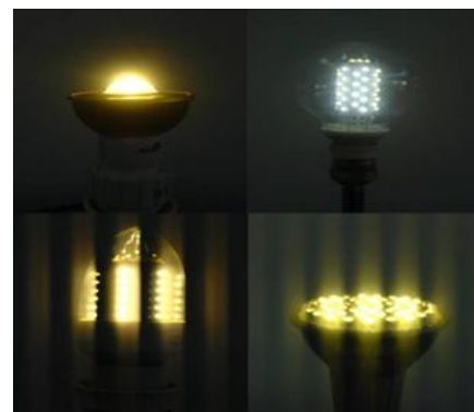
Figure 7. Some of the LED lamps tested. The top lamps showed no flickering and this is also evident by the stripe-free photographs.
