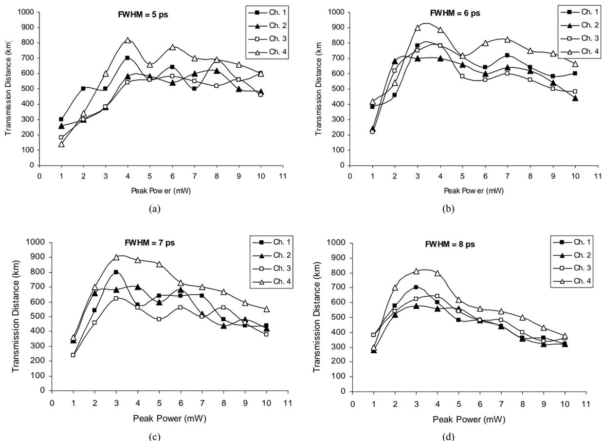
**Figure 2.** Transmission distance versus peak power for different values of FWHM: (a) 5 ps; (b) 6 ps; (c) 7 ps; and (d) 8 ps. (Channels' definitions: Ch. 1 = 1554.4 nm; Ch. 2 = 1554.8 nm; Ch. 3 = 1555.2 nm; Ch. 4 = 1555.6 nm).
