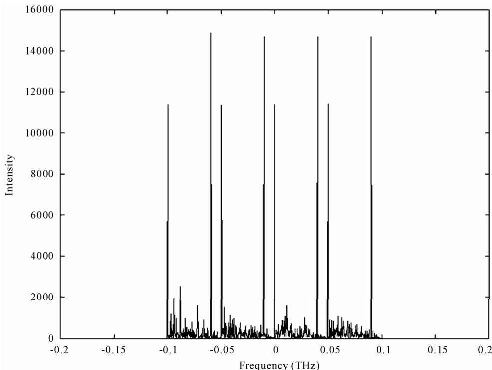
**Figure 3. Signals' spectra using Gaussian filter with 48 GHz bandwidth.**
