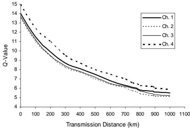
**Figure 4.**  $Q$ -value versus propagation distance for all channels using peak power = 3 mW and FWHM = 6 ps. (Channels' definitions: Ch. 1 = 1554.4 nm; Ch. 2 = 1554.8 nm; Ch. 3 = 1555.2 nm; Ch. 4 = 1555.6 nm).
