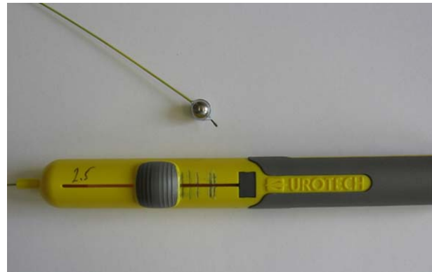
Figure 1. On the handle we established a non-linear scale in mm by grabbing standardized balls, normally used for ball bearings and standardized cylindrical steel rods for the smaller size.
