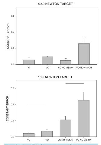
**Figure 3.** Mean + SEM for constant error. The voluntary opening prehensor had significantly higher constant error for the vision conditions (t = -2.48, p < 0.05) and the no-vision condition (t = -2.18, p < 0.05) at the 10.5 N target. Horizontal lines represent comparisons where there was a significant difference as elucidated by a t-test.
