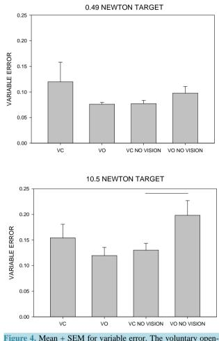
ing prehensor had significantly higher variable error. The voluntary opening prehensor had significantly higher variable error for the novision condition (t = -2.15, p < 0.05) at the 10.5 N target. Horizontal lines represent comparisons where there was a significant difference as elucidated by a t-test.
