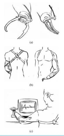
Figure 1. In (a), shows a schematic of the voluntary closing split hook prehensor (left) and voluntary opening split hook prehensor (right). In (b), shows a schematic of the cabling system and prosthetic limb of an upper extremity amputee. In (c), shows a schematic of a person with an amputation using a prosthesis performing the static grip force experiment.
