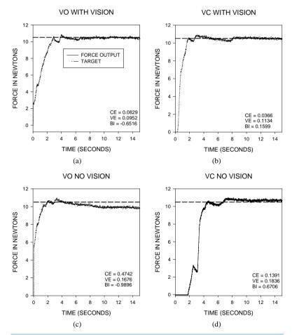
Figure 2. Examples of the force output produced by using the voluntary opening prehensor (left two panels) and the voluntary closing prehensor (right two panels). The two upper panels represent the force output for the voluntary opening and voluntary closing prehensors with vision and the lower two panels represent the force output for the voluntary opening and voluntary closing prehensors with no vision. The inset values give the corresponding CE, VE, and BI for each trial.
