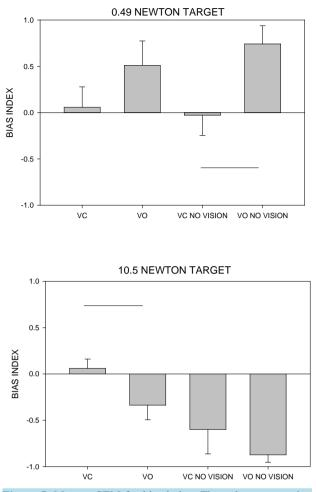
Figure 5. Mean + SEM for bias index. The voluntary opening prehensor overshot the target more than the voluntary closing prehensor for the no vision condition at the 0.49 N target (t = 2.13, p < 0.05). The voluntary opening prehensor undershot the target more than the voluntary closing prehensor for the vision condition at the 10.5 N target (t = -2.614, p < 0.05). Horizontal lines represent comparisons where there was a significant difference as elucidated by a t-test.
