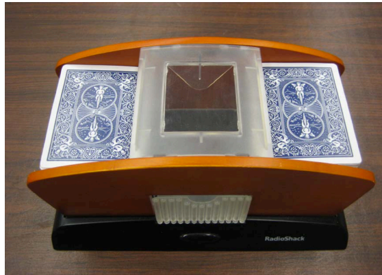
Figure 1. Motor-driven mechanical card shuffler used to generate auto-shuffled card sequences. Two piles of cards placed as shown are displaced from below by rotating wheels so as to drop sequentially into the central chamber.
