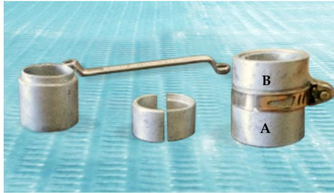
**Figure 1.** Cylindrical mould, lower ring (A) for the impression material and upper ring (B) to receive the stone material and finally the stone mould.
