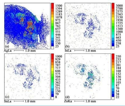
Figure 5. Electron probe microanalysis (EPMA) in Case 1: (a) The metal components were silver 69.2%; (b) indium (6.4%); (c) tin (11.3%); and (d) zinc (13.1%).
