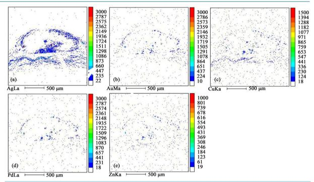
Figure 10. Electron probe microanalysis (EPMA) in Case 2: (a) The metal components were silver 61%; (b) gold (7.4%); (c) copper (10.8%); (d) palladium (9.7%); and (e) zinc (4.5%).
