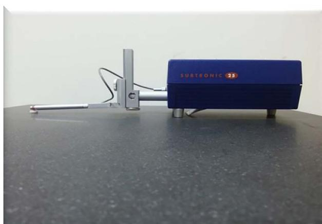
Figure 3. Testing of surface roughness with profilometer.
