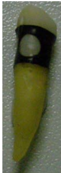
Figure 1. One of the specimens with its black rectangular piece of adhesive tape and the round opening on it to match the size of the colorimeter apparatus; the black tape was applied on the facial aspect of the crown in such a way that the round opening was positioned on the cervical third of the crown.
