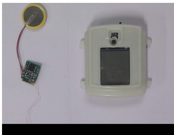
Figure 3. The monitoring circuit (18 mm × 16 mm × 5 mm) and the button battery (20 mm × 2.5 mm), and the receiver.
