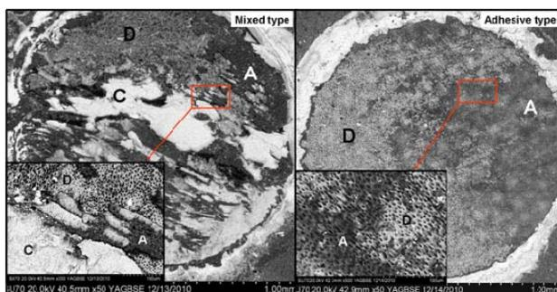
**Figure 2.** FE-SEM images in backscattered scanning electron mode at high and low magnification of “mixed-type” failure across the different interfacial layers and “adhesive” failure between dentin and adhesive (C = composite; D = dentin; A = adhesive).
