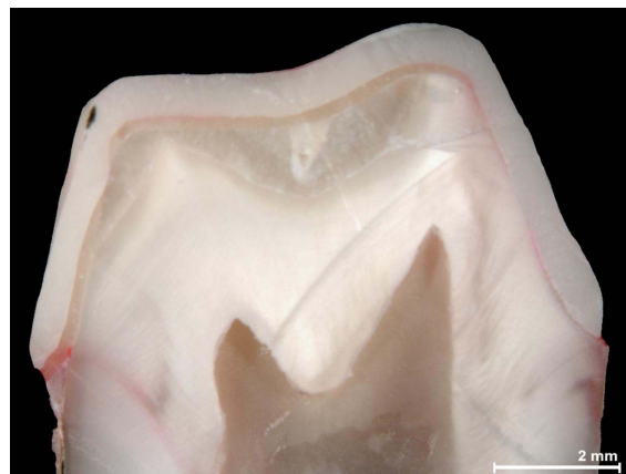
Figure 3. Representative microphotograph of microleakage detection with 2% fuchsin basic. As described in section "material and methods". The tooth section shows leakage up to two thirds of dentin. Bar represents 2 mm.
