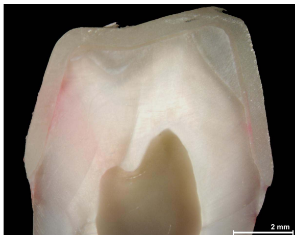
Figure 4. Representative microphotograph of microleakage detection with 2% fuchsine basic. As described in section “material and methods”. The tooth section shows leakage up to three thirds of dentin without compromise of pulp. Bar represents 2 mm.
