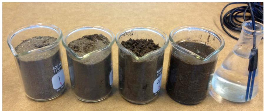
**Figure 4.** Soil and water containers used to calibrate the Decagon EC-5 sensors.
