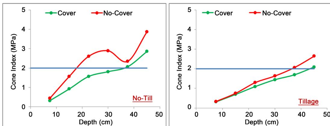
Figure 4. Effects of cool season cover crop and tillage on soil compaction.
