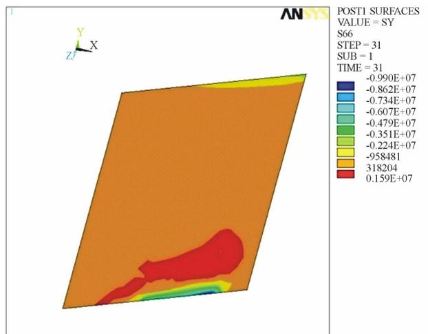
Figure 15. Stress  $S_y$  at section C-C (Pa).
