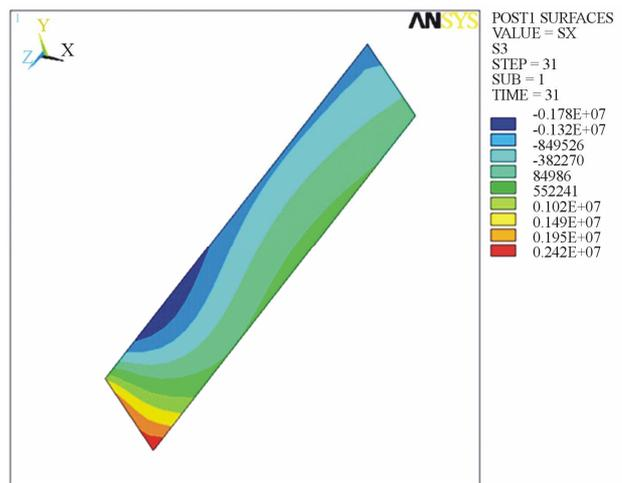
Figure 14. Stress  $S_x$  at section B-B (Pa).
