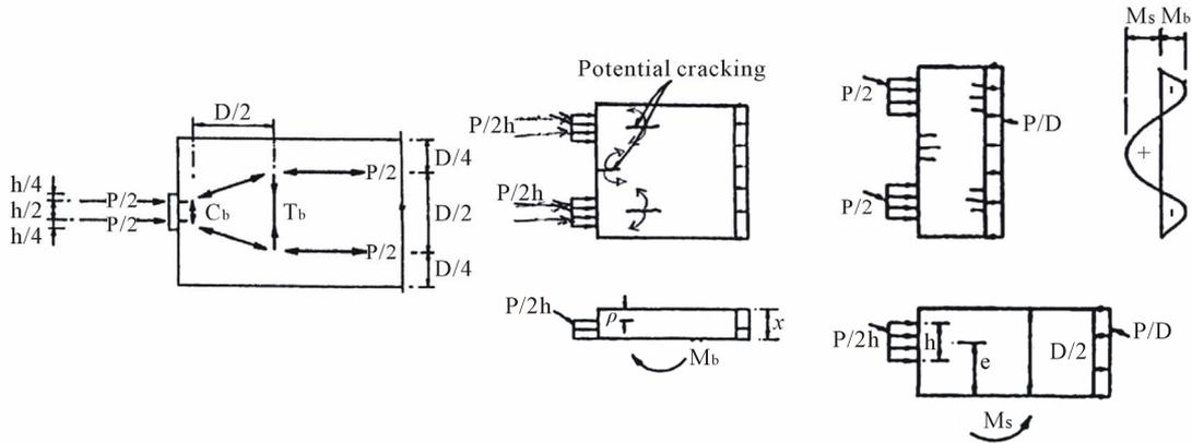
Figure 6. Analog truss for one and two concentrated loads [2].
