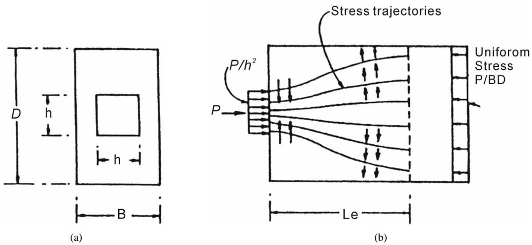
Figure 2. Contour lines of stresses for concentrated loads applied over the plane [2]. (a) End elevation; (b) Side elevation.
