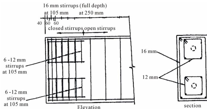
Figure 7. Typical details of reinforcements for two symmetric concentrated loads on beam [2].
