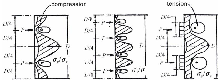
Figure 5. Transverse stress isoloads for multiple concentrated loads [2].
