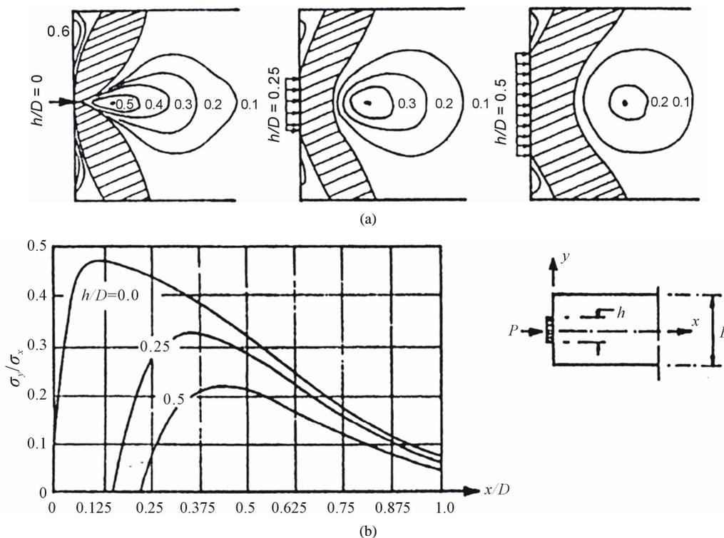
**Figure 4.** Distribution of transverse stresses for symmetric (central) concentrated loads [2]. (a) Stress Isobars ( $\sigma_y/\sigma_x$ ); (b) Transverse stress along member axis for various anchorage plate sizes.
