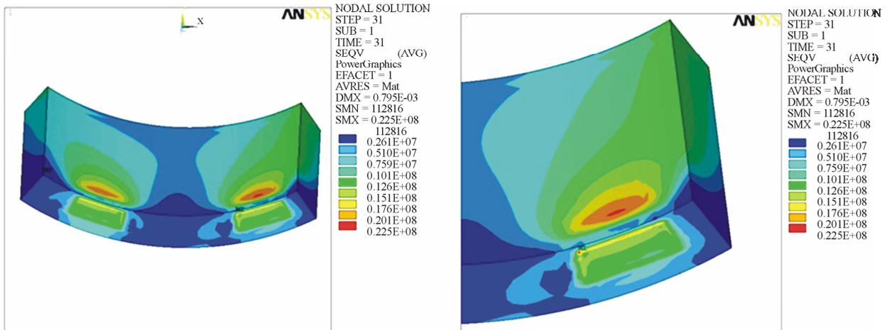
Figure 11. Von Mises stress of segment at the end of the loading (Pa).
