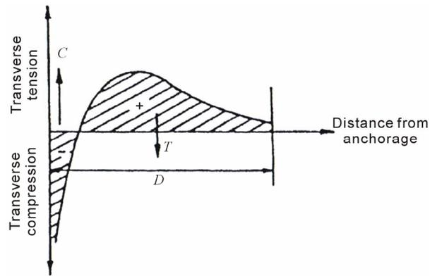
**Figure 3.** Distribution of transverse stresses beyond concentrated load [2].
