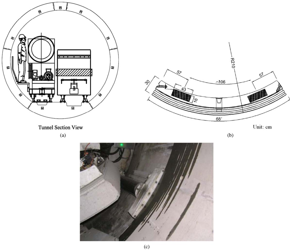
Figure 1. Application point of TBM jack loads on final lining and typical tunnel section.
