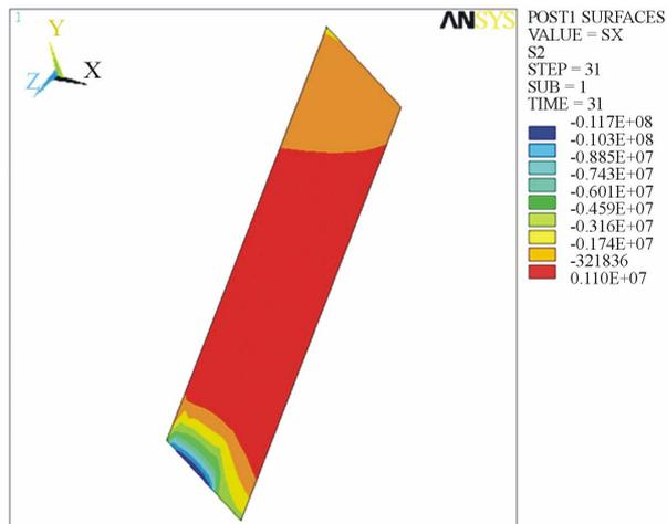
Figure 13. Stress  $S_x$  at section A-A (Pa).
