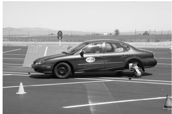
Figure 1. Sedan equipped with skid monster.
