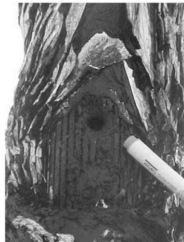
**Figure 13. Bushing failure caused by degradation of its insulation.**
