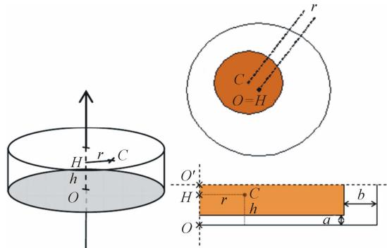
Figure 3. Parameters of interest to determine core off-center. For symmetry reasons, the left and upper parts of the transverse cut may be omitted.
