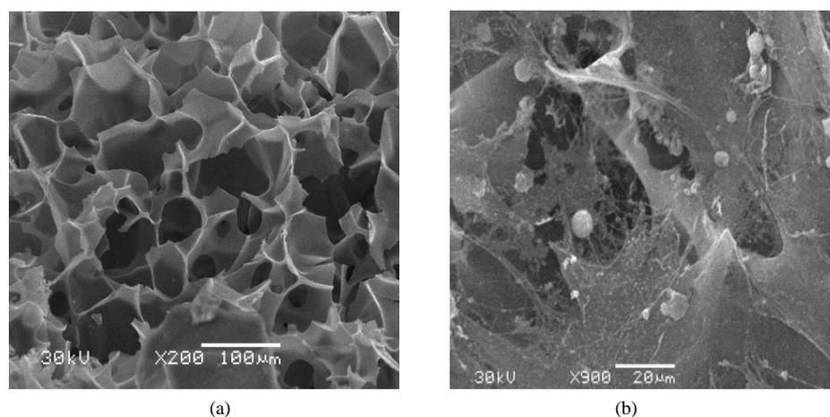
**Figure 1.** Silk fibroin scaffold under SEM, before and after coculture with hUCMSCs. (a) Silk fibroin scaffold (SEM,  $\times 200$ ); (b) Cell-scaffold complex, 2 weeks after adipogenic induction (SEM,  $\times 900$ ).
