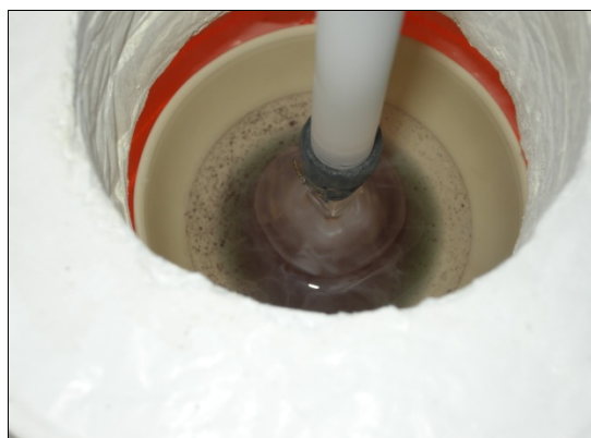
Figure 1. The single crystal KCl:Mn in growing.
