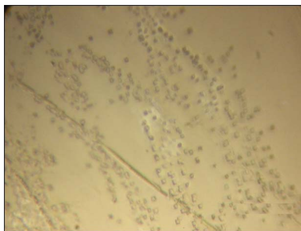
Figure 6. The picture of Etchpit from chemical etching in the surface of the crystal of KCl:Ag.
