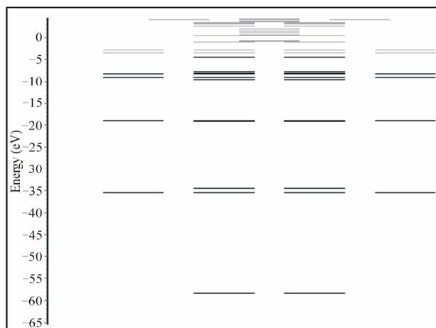
**Figure 3.** Molecular orbital diagram of  $ZrI_3$ - $ZrI_3$  triplet system at  $eq + 6.0\text{\AA}$  separation. Black indicates occupied orbitals, grey indicates virtual (unoccupied) orbitals.
