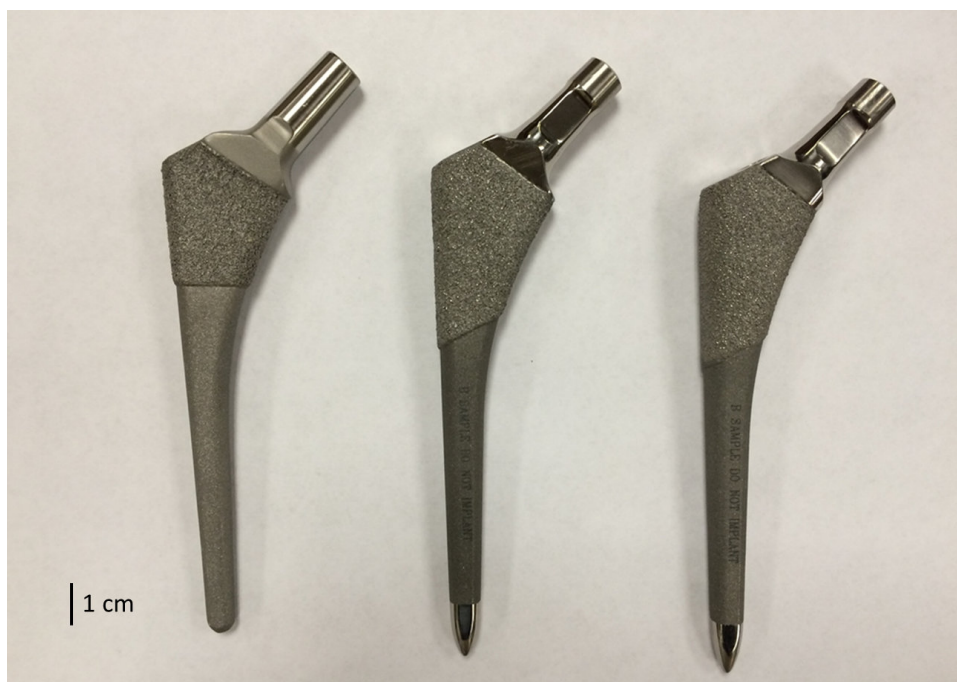
Figure 1. From left to right, Bi-Metric, Echo Bi-Metric full proximal profile (FPP), Echo Bi-Metric reduced proximal profile (RPP). Scale bar: 1 cm.
