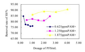
Figure 7. Flocculation effect of PAM<sup>+</sup>-PFS combination.
