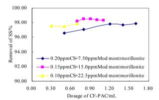
Figure 8. Flocculation effect of CS-Modified montmorillonite-CF-PAC combination.
