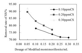
Figure 2. Flocculation effect of CS-Modified montmorillonite.
