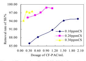
Figure 4. Flocculation effect of CS-CF-PAC combination.
