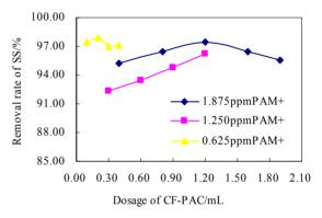
Figure 5. Flocculation effect of  $PAM^+$ -CF-PAC combination.
