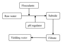
Figure 1. Experimental process.
