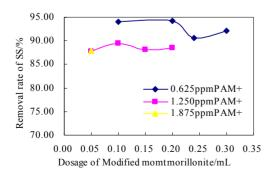
Figure 3. Flocculation effect of PAM<sup>+</sup>-Modified montmorillonite.
