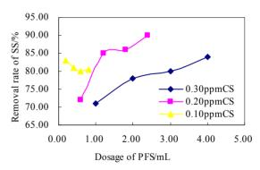
Figure 6. Flocculation effect of CS-PFS combination.
