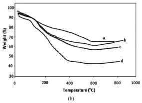
Figure 4. TGA of (a) a:  $gly_1$ , b:  $gly_3$  and c:  $gly_2/MMT$  nanocomposites; (b) a: p-St, b: p-MMA, c:  $gly_5$  and d:  $gly_4/MMT$  nanocomposites.
