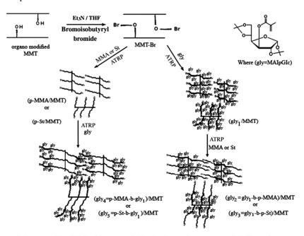
Scheme 1. SI-ATRP of homo and block glycopolymers onto MMT surface.
