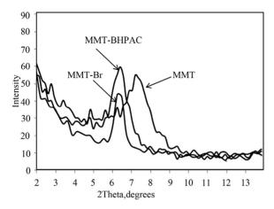
Figure 1. XRD of MMT, MMT-BHPAC and MMT-Br.
