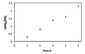
Figure 3. First order kinetic plot for SI-ATRP of gly.
