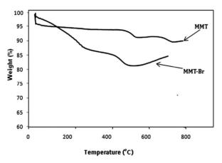
Figure 2. TGA of MMT and MMT-Br.
