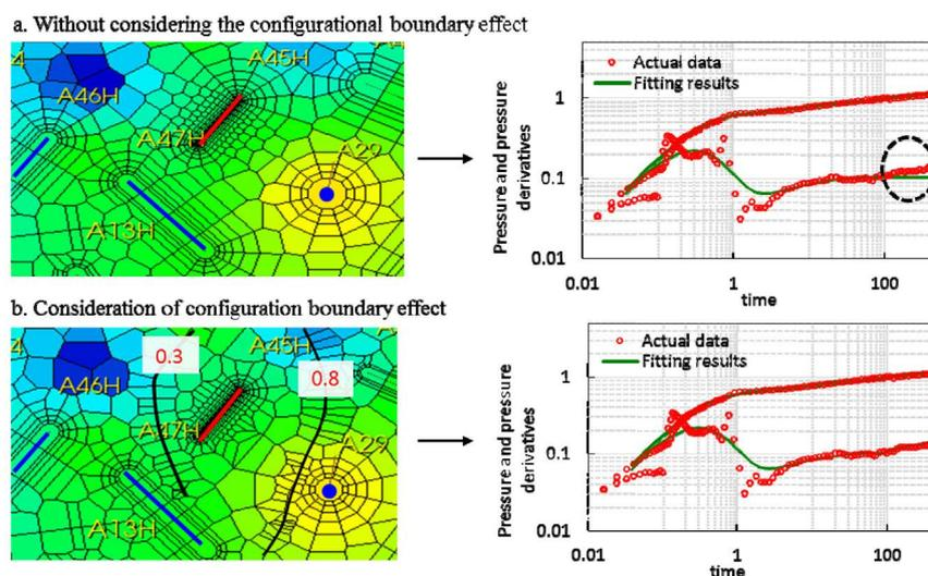
**Figure 8.** The calculation of injection-production connectivity coefficient based on pressure data of well A45H.
