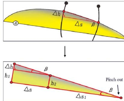
Figure 3. The theoretical calculation model for boundary of distributary sand dam.
