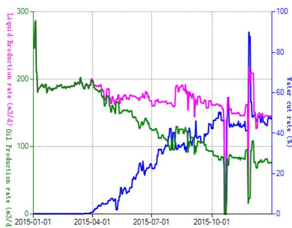
Figure 7. The production curve of Well B11H.
