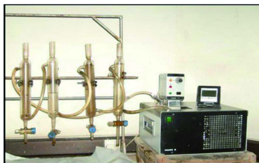
Figure 1. Water separation equipment.
