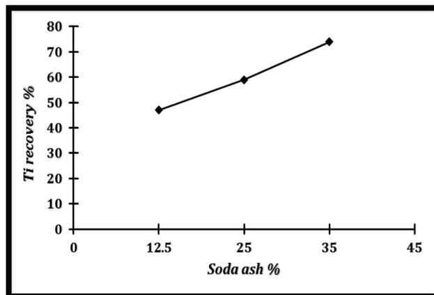
Figure 5. Relationship between the amount change of soda ash and degree of conversion of titanium oxide at 900°C for pellet samples.
