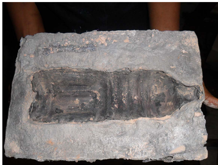
Figure 8. The finished half-mould after the incorporation of the backing layer.
