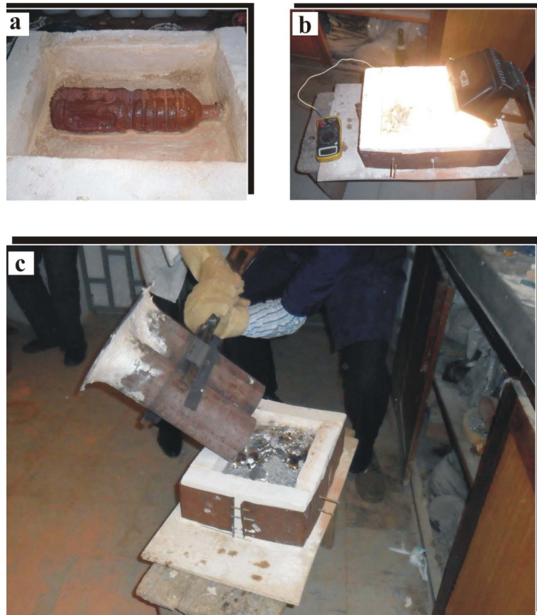
Figure 5. (a) The electroform was positioned inside an open mould; (b) The mould was preheated for about 30 min to 120°C with floodlights; (c) The molten aluminium was poured directly on top of the electroform.
