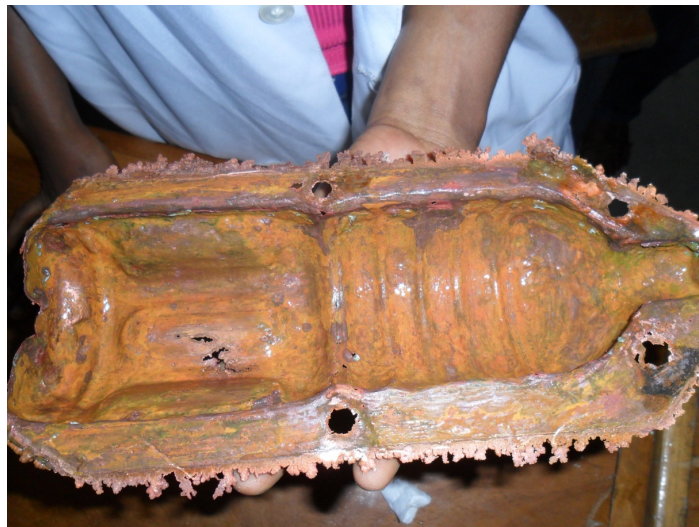
Figure 7. The interior view of the electroformed copper insert.
