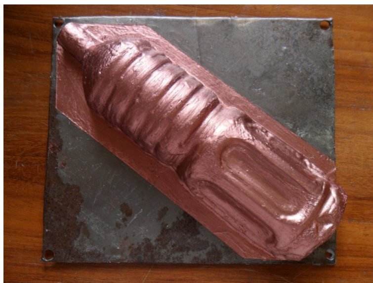
Figure 3. POP mandrel with the copper conducting paint layer applied.
