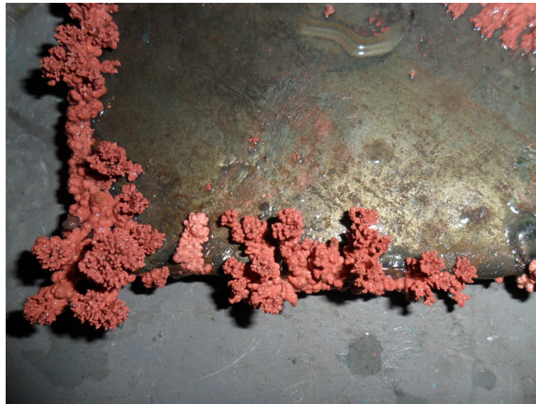
Figure 13. Parasitic growth of copper through cracks and fissures in the epoxy-coated steel base plate.
