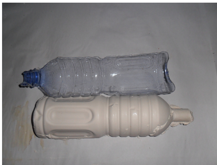
Figure 1. Longitudinally split section of the plastic bottle and the cast POP mandrel.
