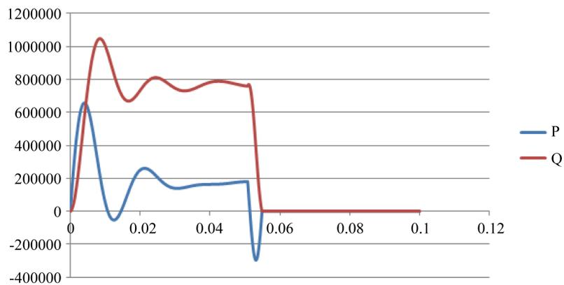
Figure 20. Active and reactive power for a wind speed equal to 27 m/s.
