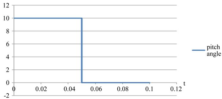
Figure 18. Variation of the pitch angle for a wind speed equal to 27 m/s.
