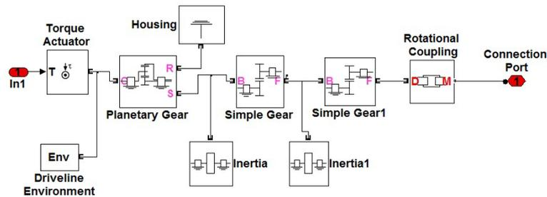
Figure 6. Model of gear train.
