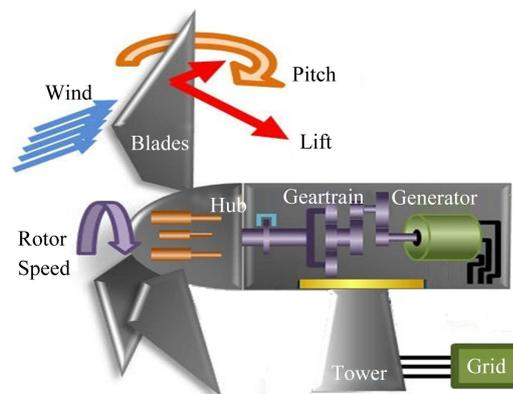
**Figure 1.** Wind turbine system [6].
