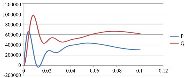
Figure 15. Active and reactive power of the wind turbine.
