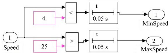
Figure 9. Model of blade protection.
