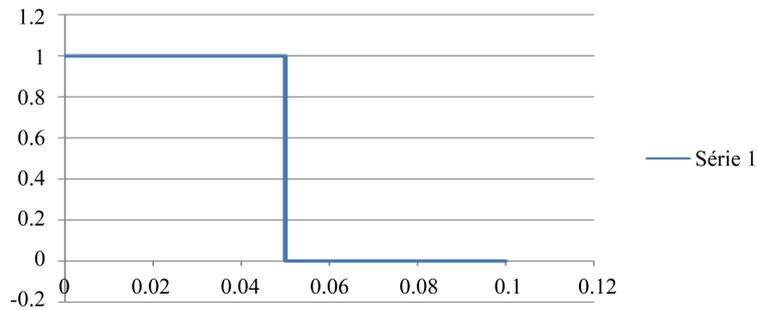
Figure 19. Variation of breaker command for a wind speed equal to 27 m/s.
