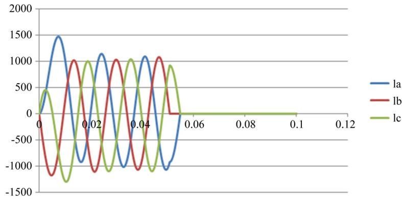
Figure 17. Currents of the wind turbine for a wind speed equal to 27 m/s.
