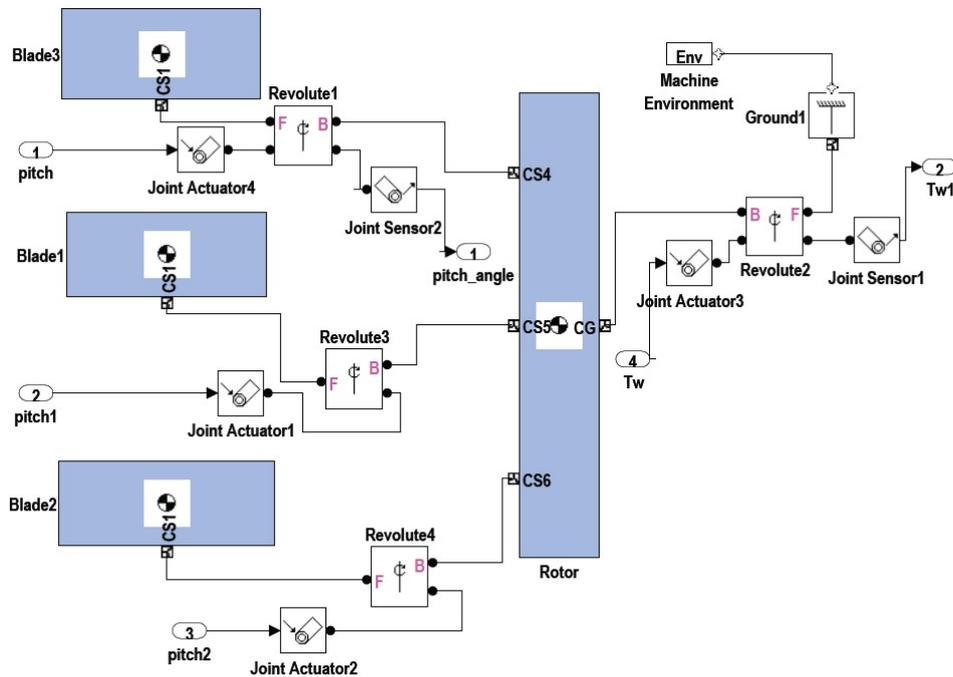
Figure 5. Model of rotor subsystem in simmechanics.
