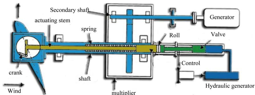
**Figure 2.** Hydraulic pitch actuator [14].
