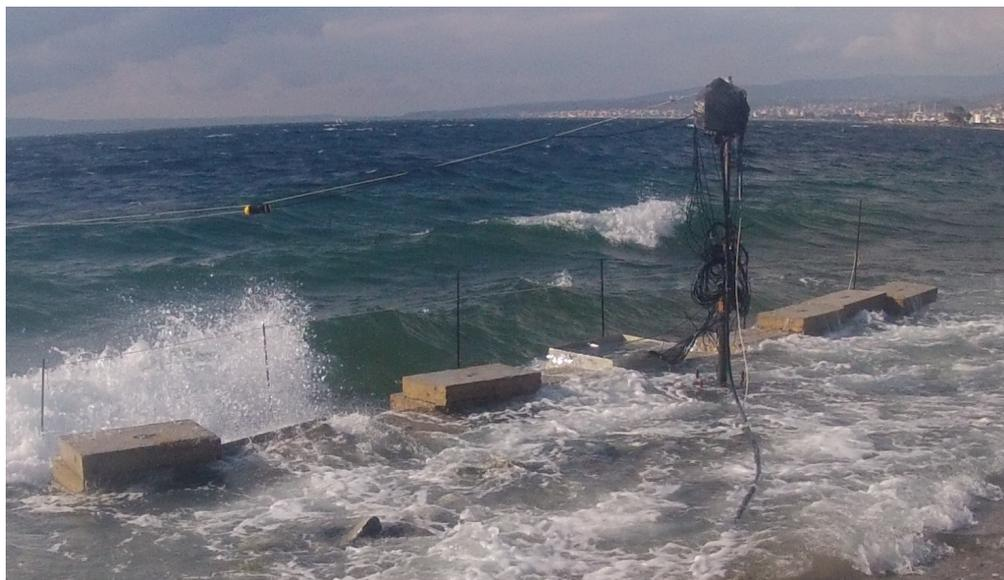
**Figure 6.** Breakwater B destroyed after 45 minutes of wind seas with the characteristics (8 - 14).
