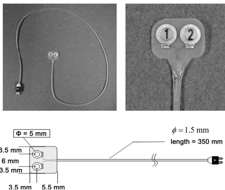
**Figure 1.** This photograph shows the new stimulation electrode for continuous vagus nerve monitoring.
