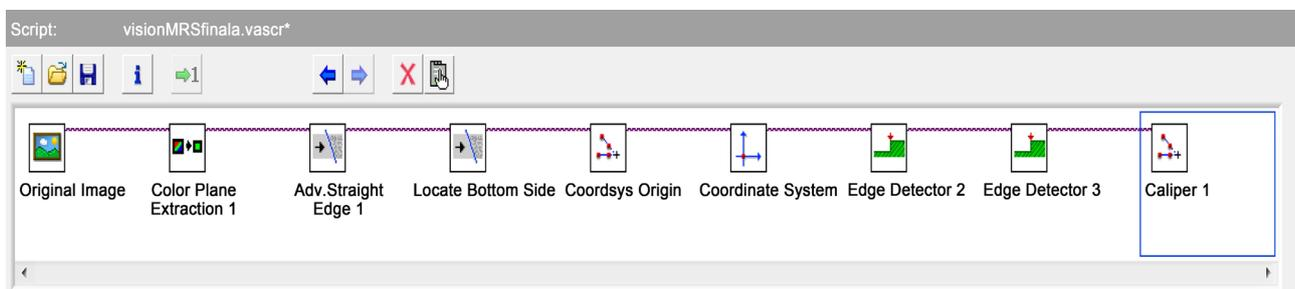
**Figure 2.** Finding height of the peaks from X-axis using vision assistant in LabVIEW.
