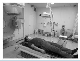
Figure 2. The experimental setup for detection of participant motion. The Kinect sensor was positioned 100cm above patient's surface.
