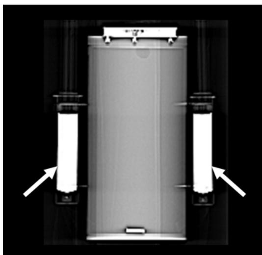
**Figure 1.** Localizer image (anterior view) of the cylindrical phantom used in this study. Two undiluted iodine syringes (arrows) were mounted beside the phantom in order to produce artifacts in the CT images.
