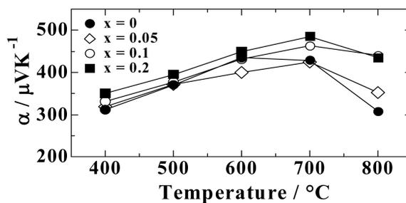
**Figure 6.** Seebeck coefficients ( $\alpha$ ) of pure and Fe-doped  $\text{YMnO}_3$  sintered bodies.
