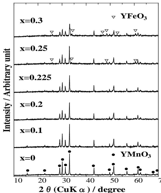
**Figure 3.** XRD patterns of calcined powders composition of which were  $\text{Y}(\text{Mn}_{1-x}\text{Fe}_x)\text{O}_3$  ( $x = 0, 0.1, 0.2, 0.225, 0.25$  and  $0.3$ ).
