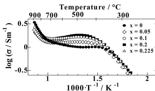
**Figure 5.** Electrical conductivity ( $\sigma$ ) of pure and Fe-doped  $\text{YMnO}_3$  sintered bodies.
