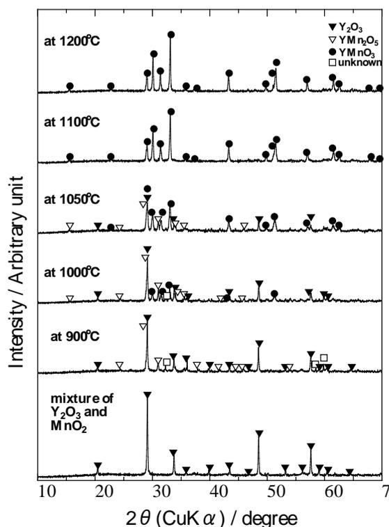
**Figure 1.** XRD patterns of powders prepared by calcination of mixed powders at temperatures between 900°C to 1200°C.
