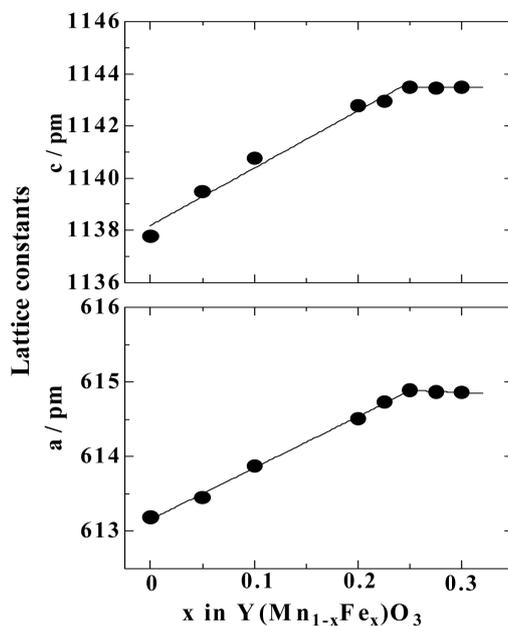
**Figure 4.** The lattice constants  $a$  and  $c$  of pure and Fe-doped  $\text{YMnO}_3$  samples.
