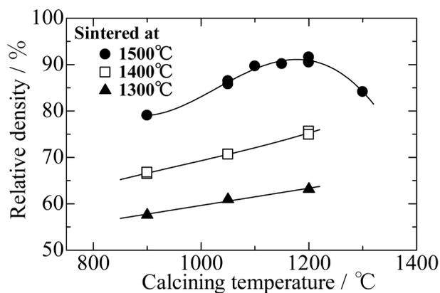
**Figure 2.** The relative densities of the sintered bodies fired at 1300°C, 1400°C or 1500°C as a function of calcining temperature of powder preparation.
