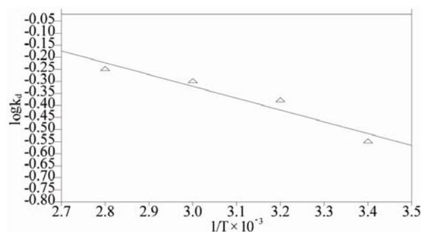
**Figure 8.** Van't Hoff plot for the sorption As(III) by MCOS. As(III): 100 mL, 410 ppb, MCOS: 0.4 g, pH:  $8 \pm 0.2$ , Contact time: 60 minutes
