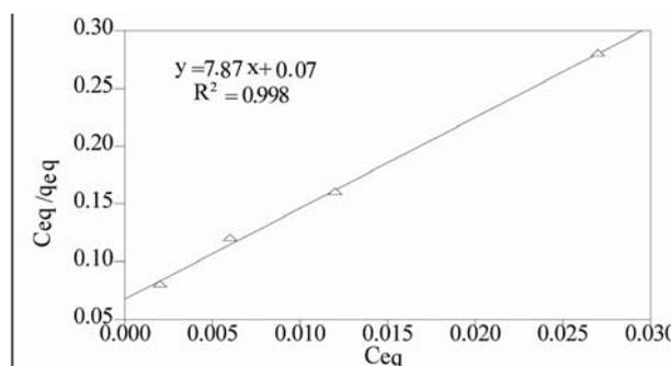
**Figure 9.** Langmuir plot for the sorption of As(III) by MCOS: 100 mL As(III), MCOS: 0.4 g, pH:  $8 \pm 0.2$ , Temperature:  $28 \pm 3^\circ\text{C}$ , Contact time: 210 minutes
