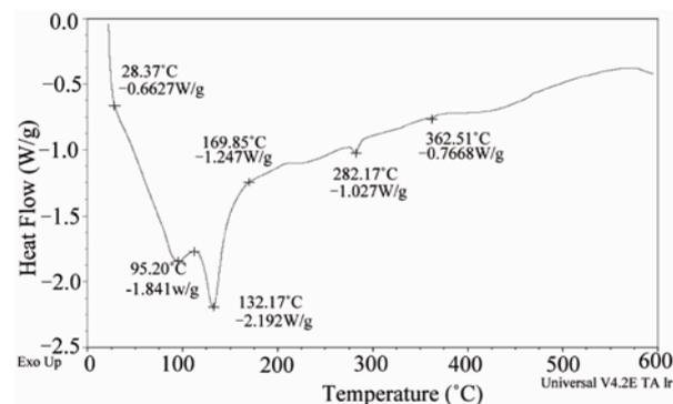
**Figure 6.** Differential Scanning Calorimetry (DSC) of MCOS at temperature 600°C.
