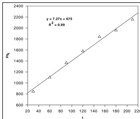
**Figure 7.** Second order kinetics for sorption of As(III) by MCOS. As(III): 100 mL, 410 ppb, MCOS: 0.4 g, pH:  $8 \pm 0.2$ , Temperature:  $28 \pm 3^\circ\text{C}$ .
