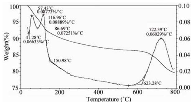
**Figure 5.** TGA-DTA Analysis of MCOS at temperature 800°C.
