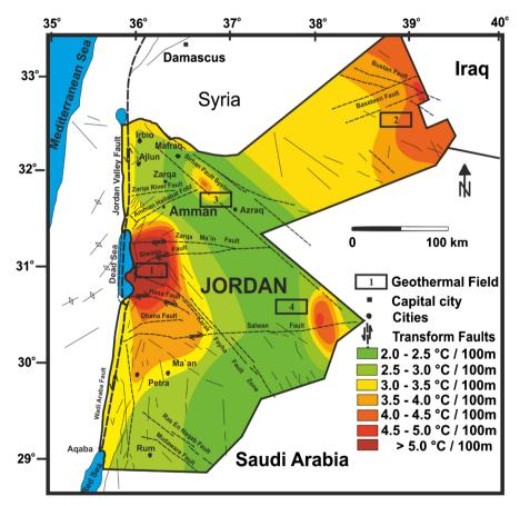
**Figure 1.** Jordan updated geothermal gradient map indicates four main geothermal fields (after [18] [19] and [20]; Structural map of Jordan (after [21] and [22]).
