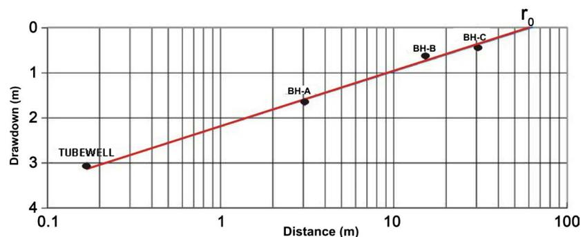
**Figure 5.** Distance drawdown graph of pumped well.
