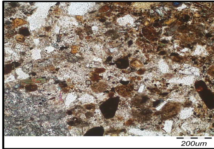
Figure 22. Thin section photomicrograph of the sample submitted by Double wall filler mortar (XPL, 10).
