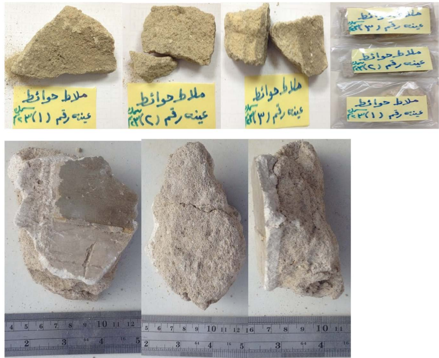
Figure 26. Some collected plaster samples.
