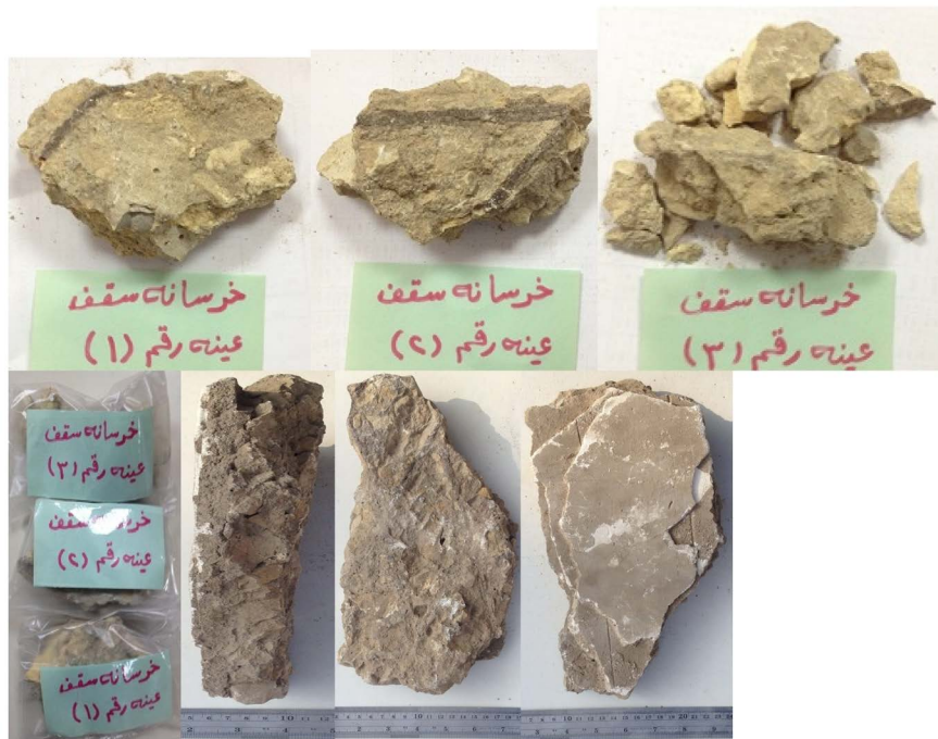
Figure 28. Collected samples from the concrete plaster samples.
