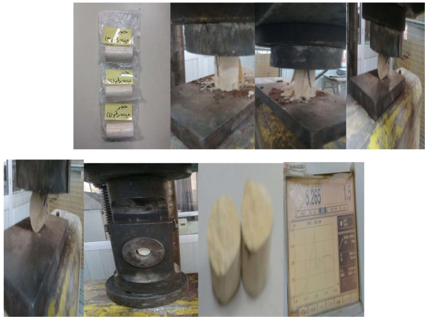
Figure 21. Mechanical testing set-up for the limestone samples.
