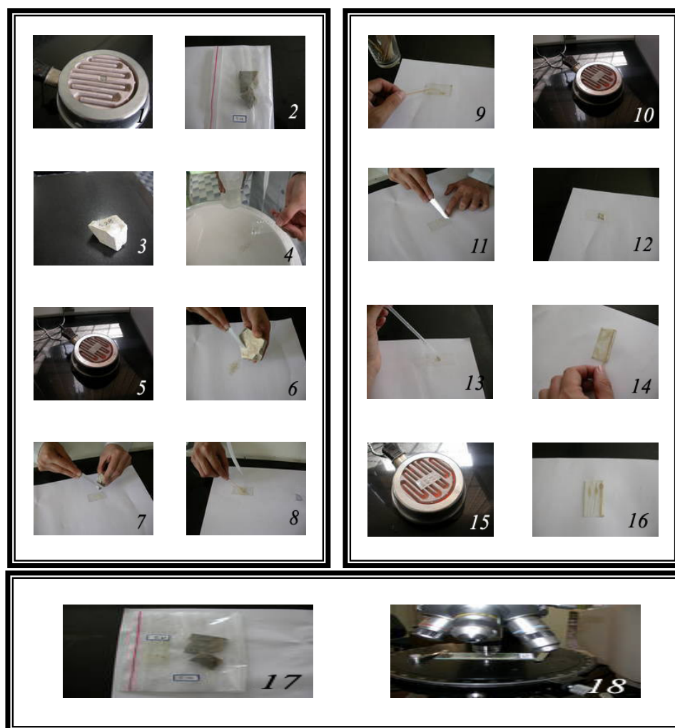
Figure 4. Preparation process microscopic sections, to the method smear slide.
