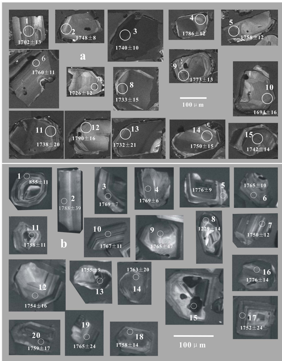
Figure 4. CL photos of zircons from Hai Zi Bimodal Intrusive rocks (a) Granite porphyry; (b) Diabase 3 U-Pb Chronological characteristics of zircon.
