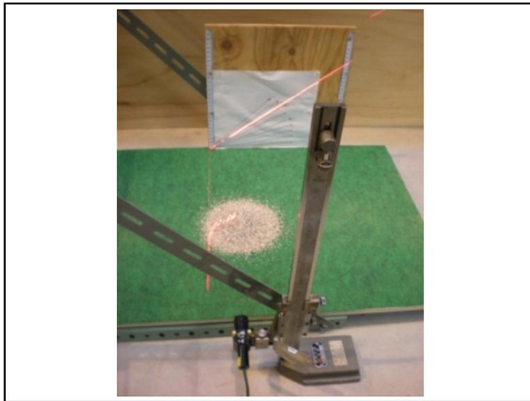
**Figure 10.** Process to measure the repose angle.
