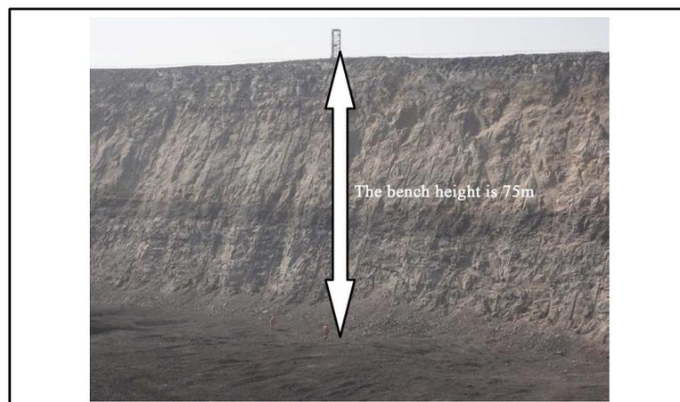
**Figure 7.** High working slope bench in a dragline operation.
