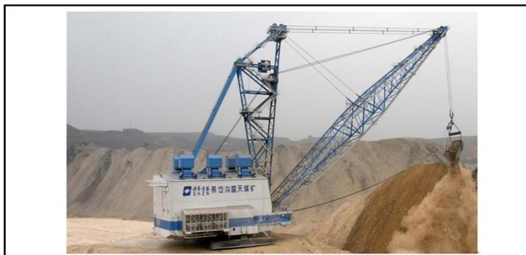
**Figure 5.** Dragline dumping operation in the internal dumping area.
