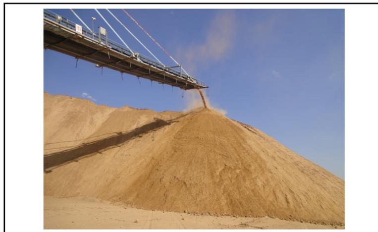
**Figure 3.** Bucket wheel excavator-belt-stacker dumping operation in the dumping area.
