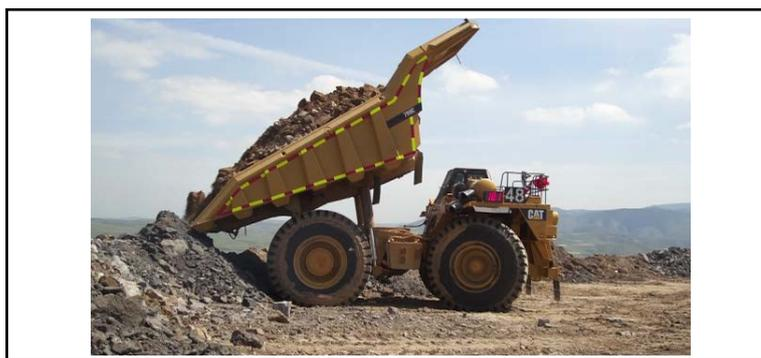
**Figure 4.** Shovel-truck-bulldozer dumping operation in the internal dumping area.
